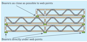
It is recommend that completed Posi-Joists be strapped together and wrapped in a waterproof protective covering to protect them from short term exposure to inclement weather.
