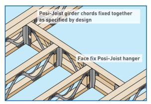
Do not notch Posi-Joist bottom chord over flange of hanger
